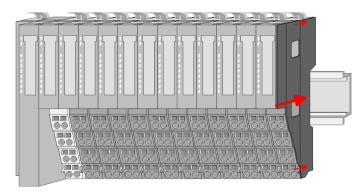
After mounting the whole system, to protect the backplane bus connectors at the last module you have to mount the bus cover, now.
