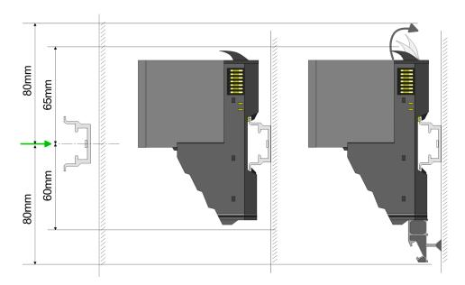
Mount the mounting rail! Please consider that a clearance from the middle of the mounting rail of at least 80mm above and 60mm below, respectively 80mm by deployment of shield bus carriers, exist.
