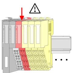
Mounting the bus cover at a peripheral module
