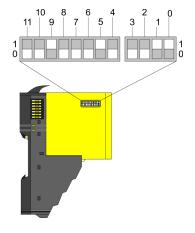
The F-address is to be configured by the F-address switch at the VIPA safety module and additionally in the master system e.g. hardware configurator. The F-address is to be set by the F-address switch besides on the safety module. Only if the F-address set in the hardware configurator accords to the setting of the F-address switch, it is possible to operate!
