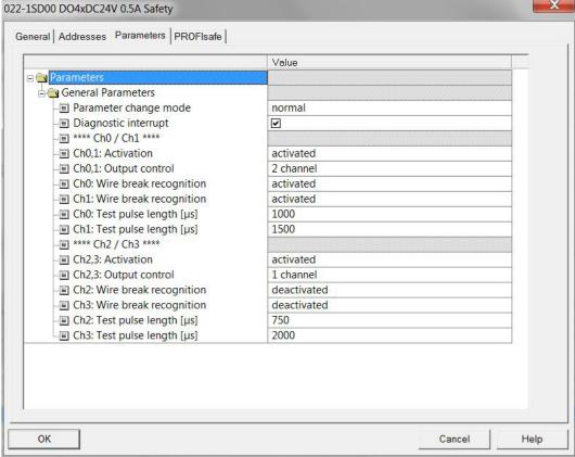
Sample application > Configuration in the Siemens SIMATIC Manager
