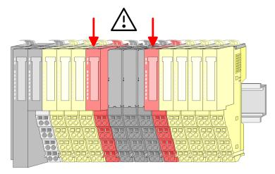
Please consider when planning with System SLIO safety modules that you may not install a System SLIO safety module behind a slave extension module of the System SLIO line extension!
