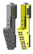
The *terminal* module serves to carry the electronic module, contains the backplane bus with power supply for the electronic, the DC 24V power section supply and the staircase-shaped terminal for wiring. Additionally the terminal module has a locking system for fixing at a mounting rail. By means of this locking system your SLIO system may be assembled outside of your switchgear cabinet to be later mounted there as whole system.
