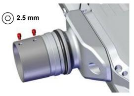
8. Route all of the required cable lines through the tube adapter and the tube.
