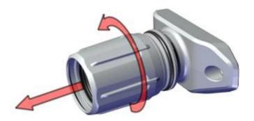
4. Apply a suitable **lubricant** to the seal and the tube end to make it easier to slide on the sealing sleeve (e.g. soap or fitting grease, depending on the application type).
