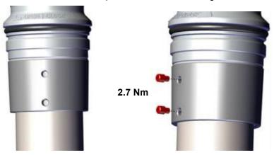
11. Lubricate the upper seal with a <u>thin</u> layer of a suitable **lubricant** (e.g. soap, fitting grease or penetrating oil, depending on the application).
