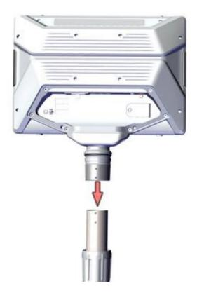
10. Align all of the parts so that the holes in the tube and in the tube adapter are positioned on top of one another and the threaded pins can be screwed in again.
