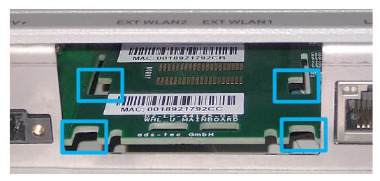
... and finally, **pushed onto the circuit board**, where they will click into place with a slight pressure. For the purposes of illustration, this image shows the back of the circuit board (usually not visible) with the metal brackets fully inserted:
