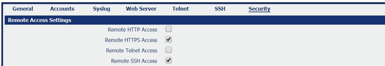
The screenshot shows a configuration interface with a top navigation bar containing tabs: General, Accounts, Syslog, Web Server, Telnet, SSH, and Security. Below the navigation bar is a dark blue header labeled "Remote Access Settings". The main content area shows four settings, each with a checkbox: "Remote HTTP Access" (unchecked), "Remote HTTPS Access" (checked), "Remote Telnet Access" (unchecked), and "Remote SSH Access" (checked).
