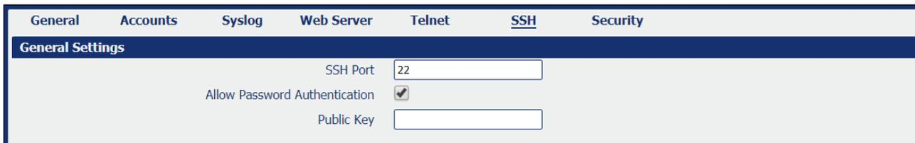
The screenshot shows a configuration interface with a top navigation bar containing tabs: General, Accounts, Syslog, Web Server, Telnet, SSH, and Security. Below the navigation bar is a dark blue header labeled "General Settings". The main content area shows three settings: "SSH Port" with a text input field containing "22", "Allow Password Authentication" with a checked checkbox, and "Public Key" with an empty text input field.
