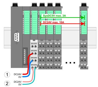
1 DC 24V for power section supply I/O area (max. 10A)
