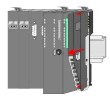
**1.** Before mounting the periphery modules you have to remove the bus cover at the right side of the CPU by pulling it forward. Keep the cover for later mounting.
