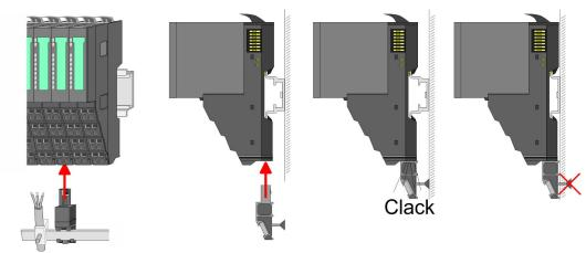
Attach the cables with the accordingly stripped cable screen and fix it by the shield 3. clamp with the shield bus.
