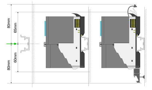
**1.** Mount the mounting rail! Please consider that a clearance from the middle of the mounting rail of at least 80mm above and 60mm below, respectively 80mm by deployment of shield bus carriers, exist.
