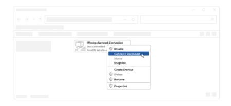
5. Choose the wireless network RUTX50 \*\*\*\* from the list and click Connect. Enter the WiFi password located on the device's label.
