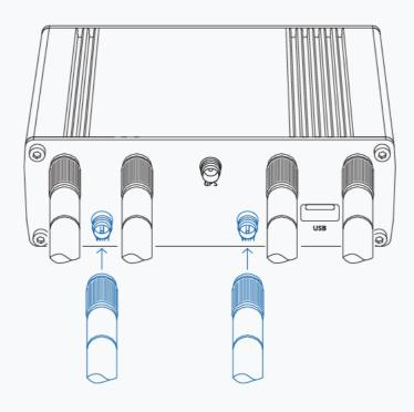
9. Power up the router by plugging in 4-pin connector to the socket in the router, and plugging adapter into electric outlet.
