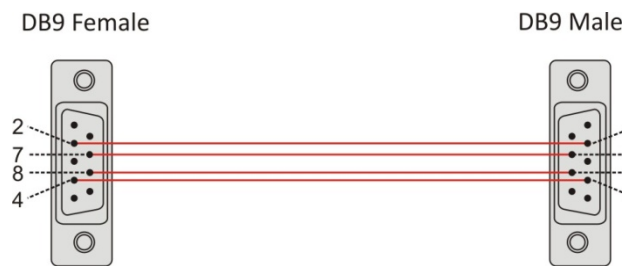
Fig. 26 – Building an extension cable
