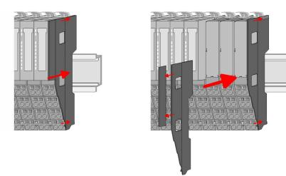
After mounting the whole system, to protect the backplane bus connectors at the last module you have to mount the bus cover, now. If the last module is a clamp module, for adaptation the upper part of the bus cover is to be removed.
