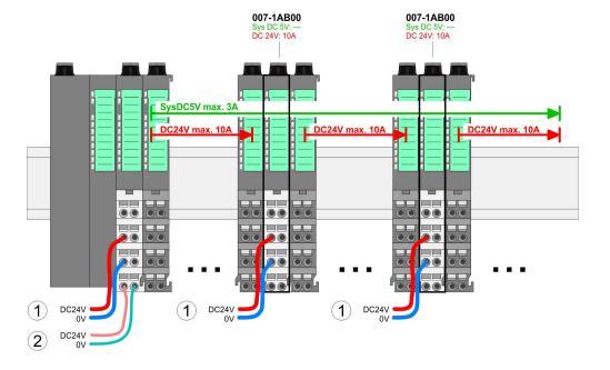
Wiring > Wiring power modules
